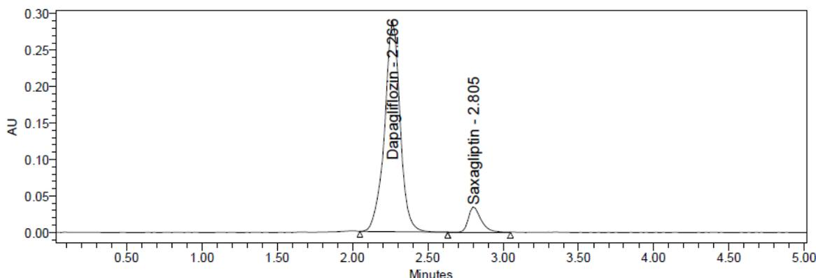
**Figure-3:** Optimized Chromatogram of Dapagliflozin and Saxagliptin
